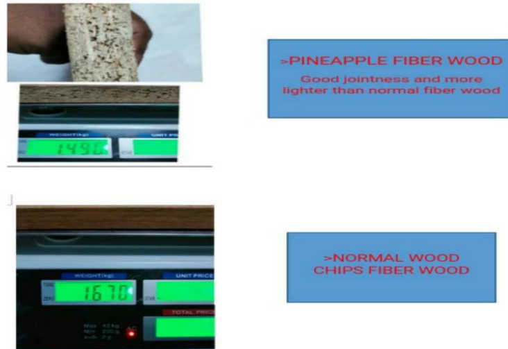
Figure 4.1 : The result for pineapple fibre wood and normal fibre wood's weight.
