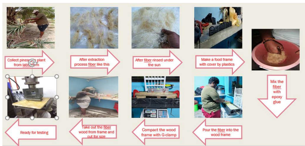
Figure 3.1 Procedure Preparation of Pineapple Fibre Wood
